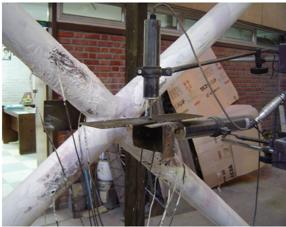
Fig. 13: LVDTs No. 17-19, strain gages 52-59, 68-71
