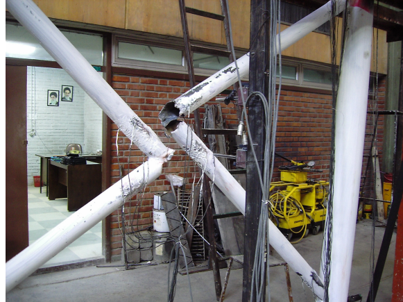
Fig. 15: Disconnection of x braces in later cycles
